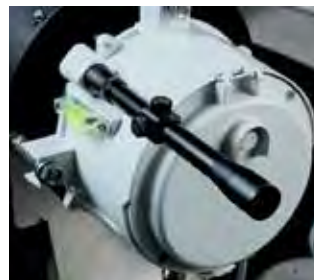
Precision alignment A gun sight can be utilized for precision alignment to the center line of the range.
