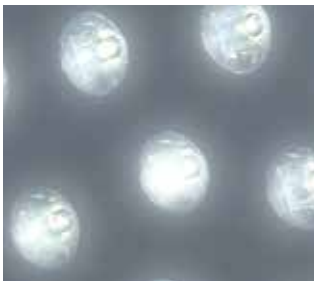
High power LEDs The performance of the range light has been achieved thanks to high power LEDs with individual lenses.
